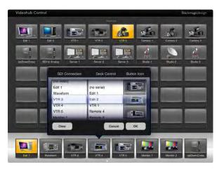
The Videohub Button Setup window allows you to set the SDI input or output connection, RS-422 deck control and the icon for the pushbutton.
