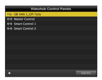
GPI and Tally Interface connected via USB
